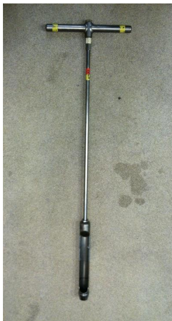
Figure 12: Typical soil probe to collect 15cm samples
