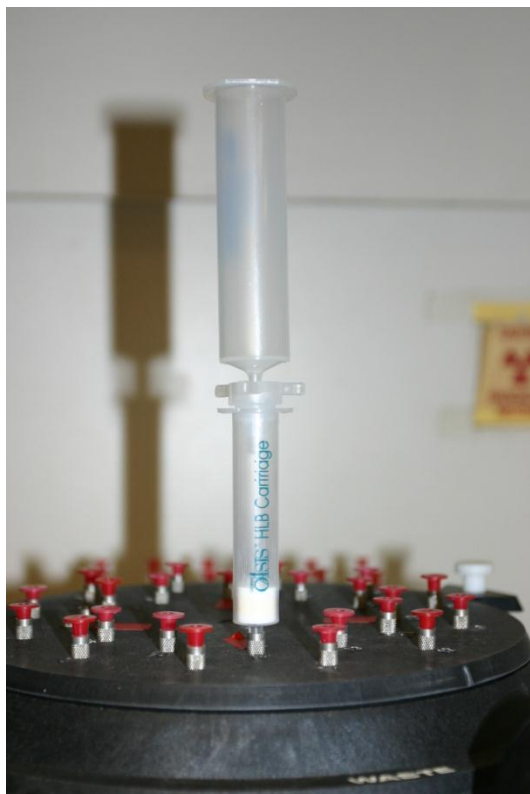
Figure 17: Oasis HLB SPE cartridge, adapter and reservoir mounted on the round vacuum unit used for cartridge conditioning and sample loading.
